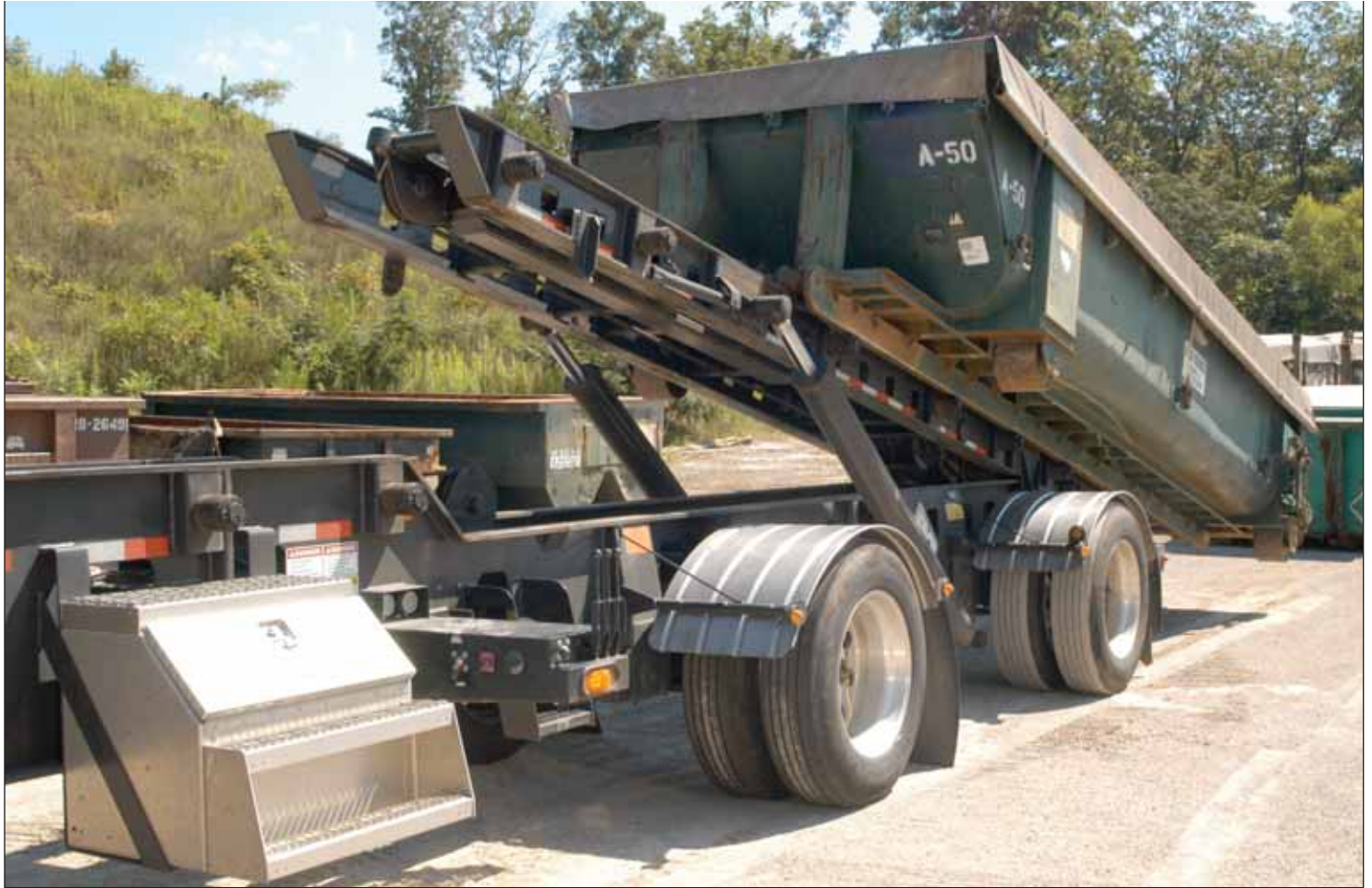
The company offers an extensive mix of specialty trailers for hazmat hauling. Above, a dumpster is loaded onto a double-bunk, roll-off chassis.
